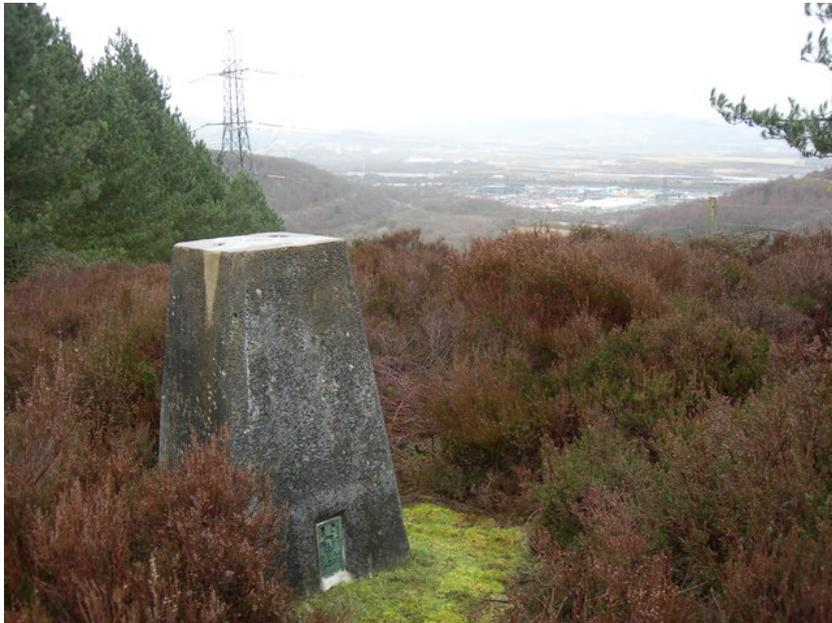
*Coed-Y-Iarll 4th Order Triangulation Pillar carries Flush Bracket S4287 which marks a point 86.121m above mean sea level.*
